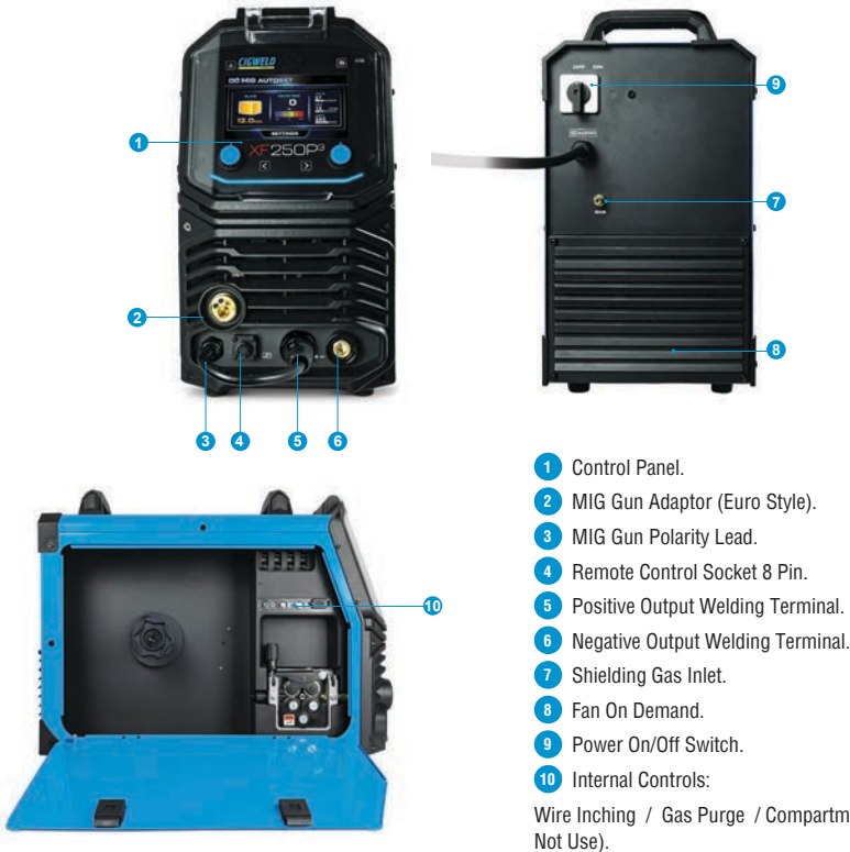
Figure 4-1: Power Source Controls, Indicators and Features
