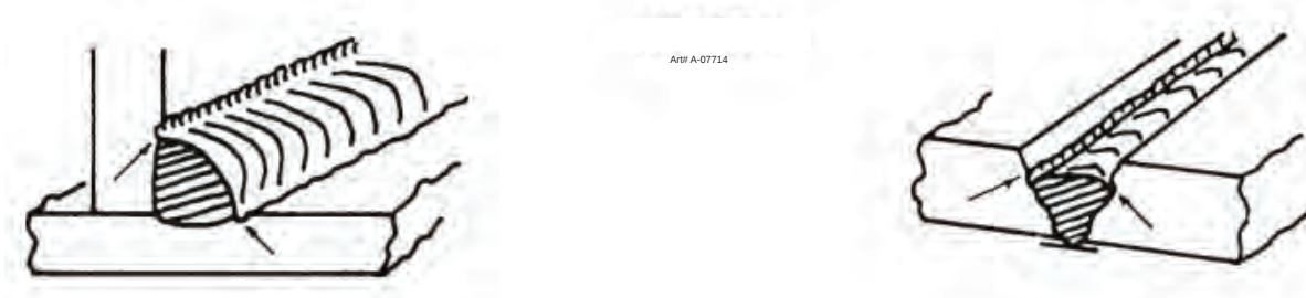
Figure 7-13: Examples of undercut
