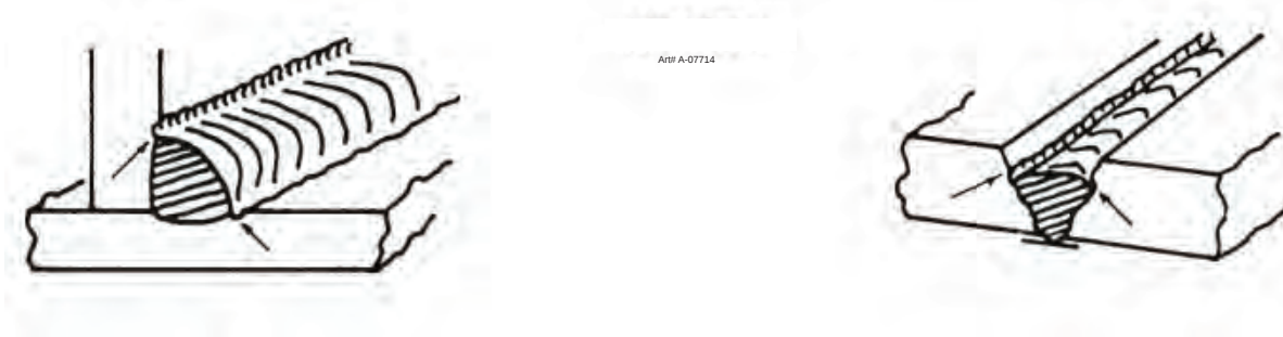
Figure 7-13: Examples of undercut
