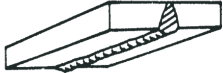
Figure 7-9: Overhead position, butt weld
