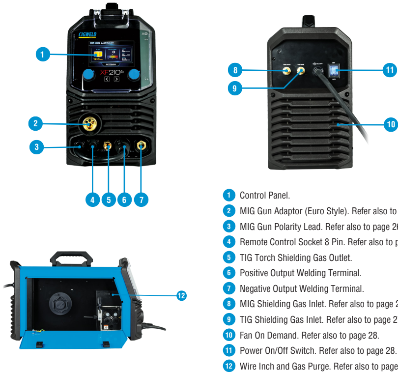
Figure 4-1: Power Source Controls, Indicators and Features
