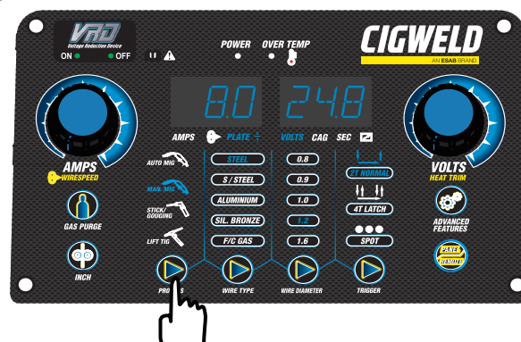
Figure 5-21: Select Manual MIG Set Mode
