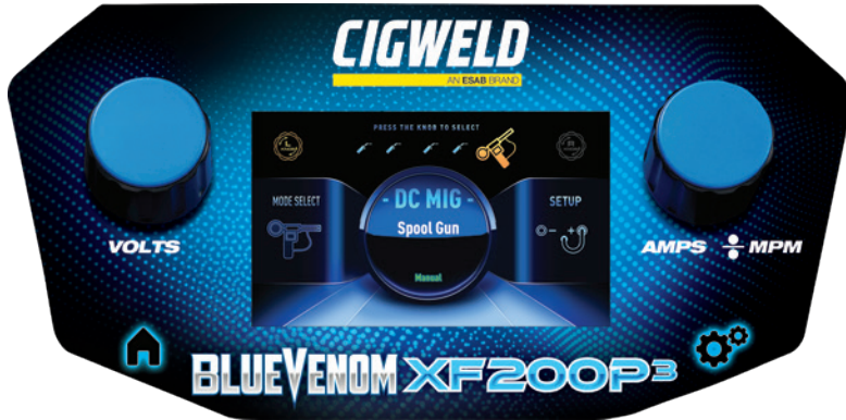
Figure 5-21: MIG (GMAW) Manual Mode And Setup With Spool Gun For Gas Shielded MIG Wire
