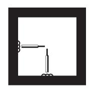
Downhand & Horizontal surfacing applications: - 3.2mm and 4.0mm sizes can be used for vertical welding by depositing overlapping horizontal stringer passes.
