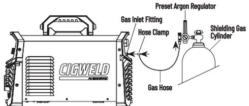
Figure 6-2: Shielding Gas Connection
