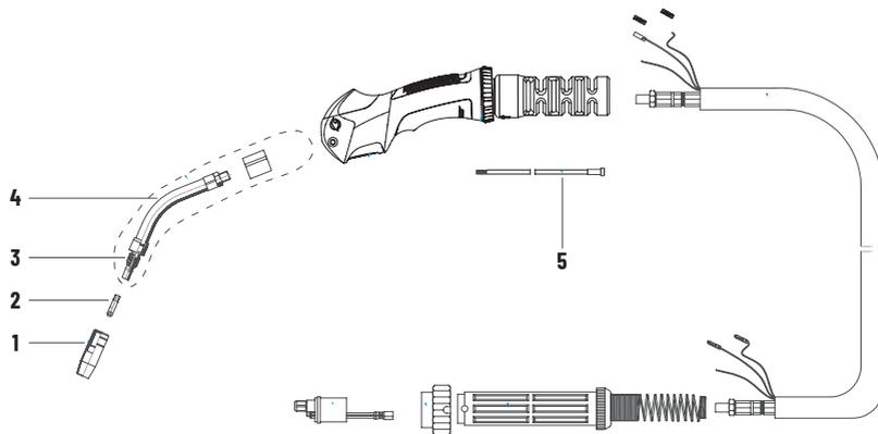
Figure 9-2: CMGBZ15E3 MIG Gun BZ15 Euro, 3m, Spare Parts
