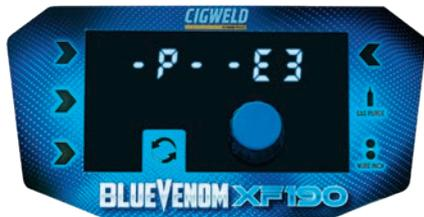
Figure 8-3: Wirefeed Motor Overload
