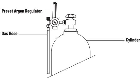
Figure 5-2: Fit Regulator/flowmeter to Cylinder
