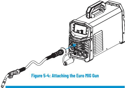
Figure 5-4: Attaching the Euro MIG Gun
