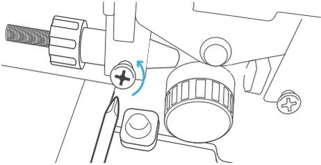
**B.** Remove the Steel Inlet Guide as fitted to the machine from factory from the Wire Drive Assembly.
