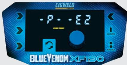
Figure 8-2: Over Temperature
