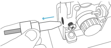
**C.** Fit the Nylon Inlet Guide into the Wire Drive Assembly as shown and tighten the retaining screw.
