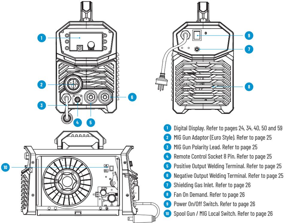
Figure 4-1: Power Source Controls, Indicators and Features
