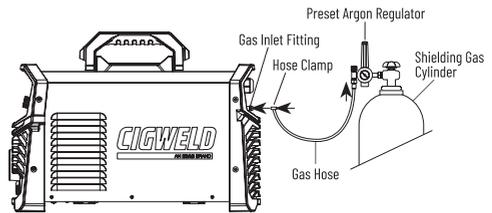
Figure 5-1: Shielding Gas Connection
