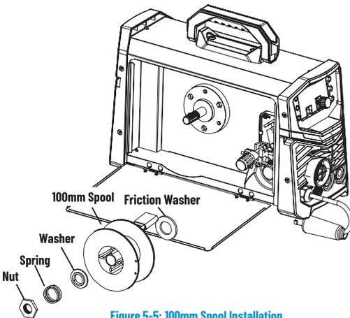
Figure 5-5: 100mm Spool Installation
