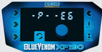
Figure 8-4: Output Over Current
