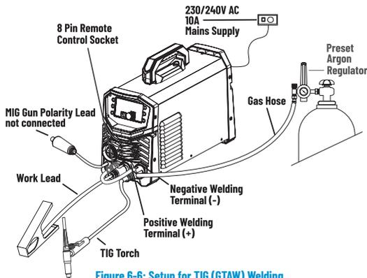
Figure 6-6: Setup for TIG (GTAW) Welding
