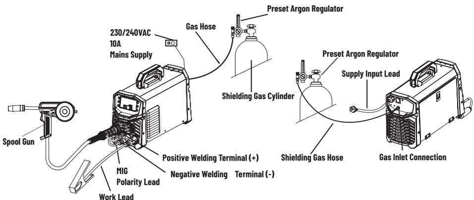
Figure 5-25: Setup with Spool Gun for Gas Shielded MIG Wire
