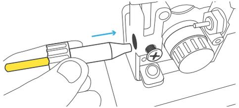
**D.** Fit the appropriate feed roll to suit the soft wire being used. Refer to sections 5.09 Changing Feed Roll and section 2.11 Optional Accessories.
