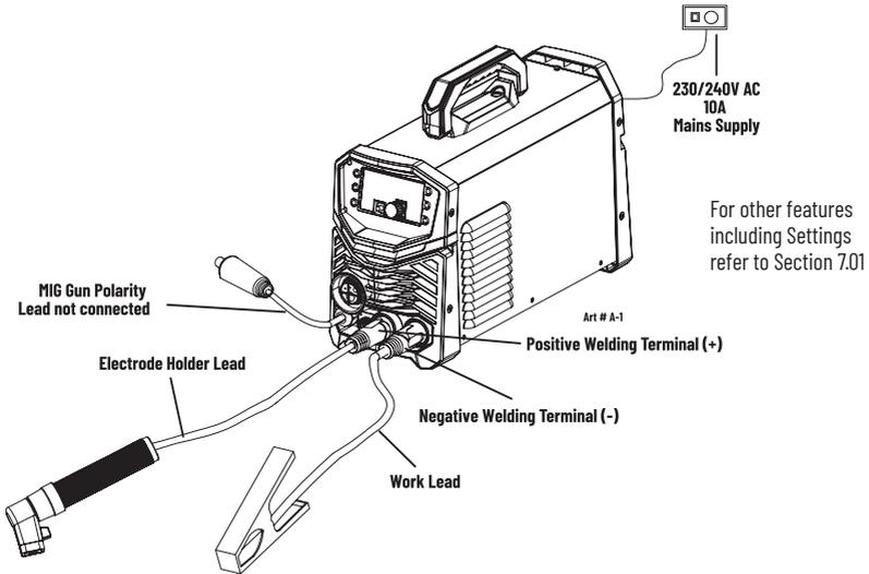
Figure 7-5: Setup for MMA (STICK) Welding
