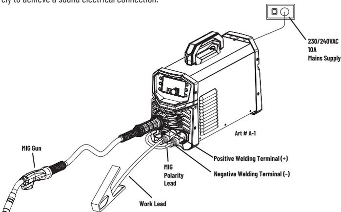
Figure 5-21: Setup for QuickSet MIG Welding with Gasless MIG Wire
