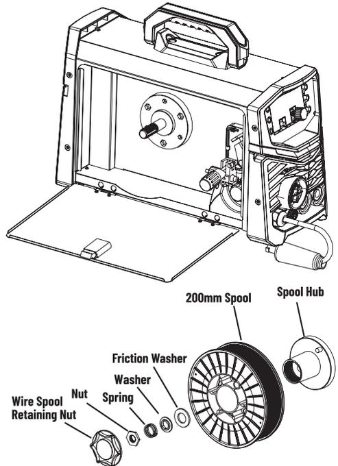
Figure 5-6: 200mm Handispool Installation
