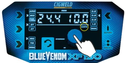
Figure 5-18: Select Wire Feed Speed Control
