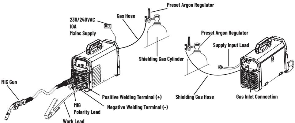
Figure 5-20: Setup for QuickSet MIG Welding with Gas Shielded MIG Wire
