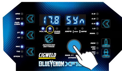
Figure 5-19: Select to Display Pre-set Volts & Trim Value
