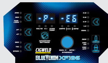
Figure 8-4: Output Over Current
