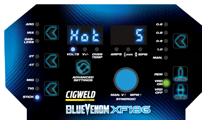
Figure 7-2: Hot Start Adjustment
