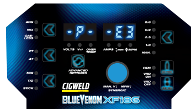
Figure 8-3: Wirefeed Motor Overload
