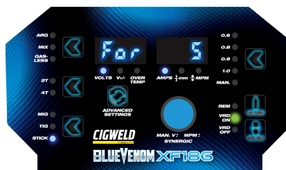
Figure 7-3: Arc Force Adjustment
