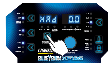
Figure 5-17: Select and Set Hard Start Value
