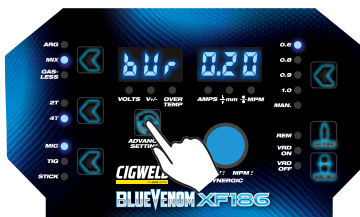
Figure 5-15: Select and Set Burnback Control Value
