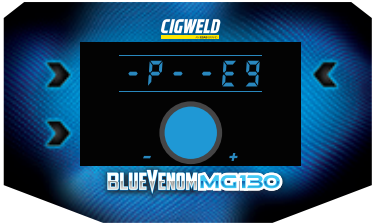
Figure 6-6: Thermal Protection Circuit Error
