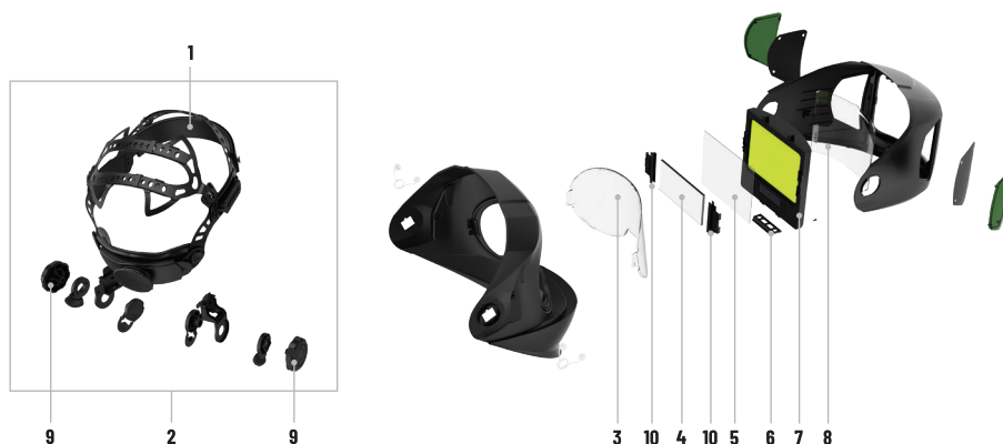
Figure 11-2 Exploded View of ArcMaster Auto-Darkening Welding Helmet
