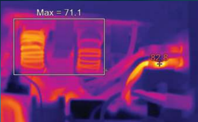
Internal thermal photo of 130 machine during use.
