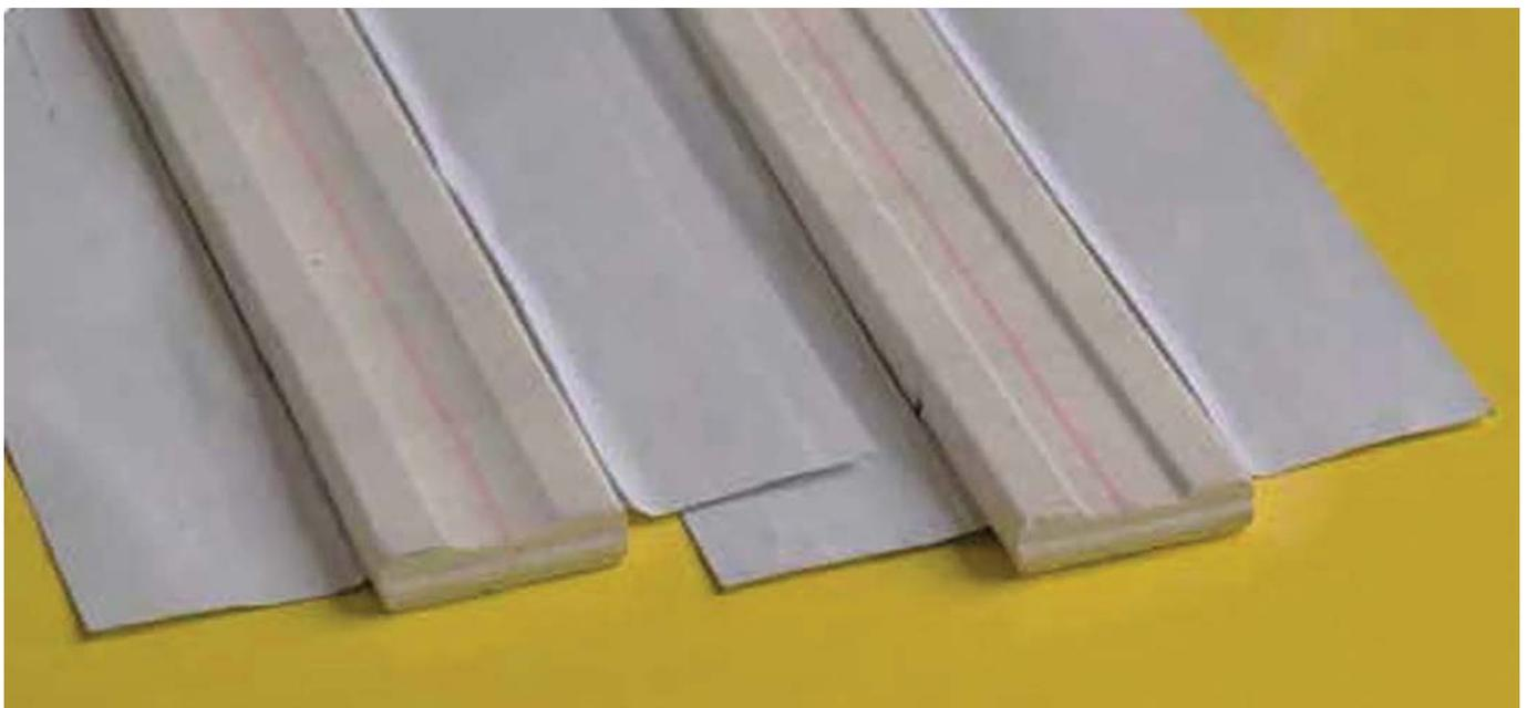
*Fastening the ceramic backing under the sheet metal using self-adhesive aluminium foil.*
