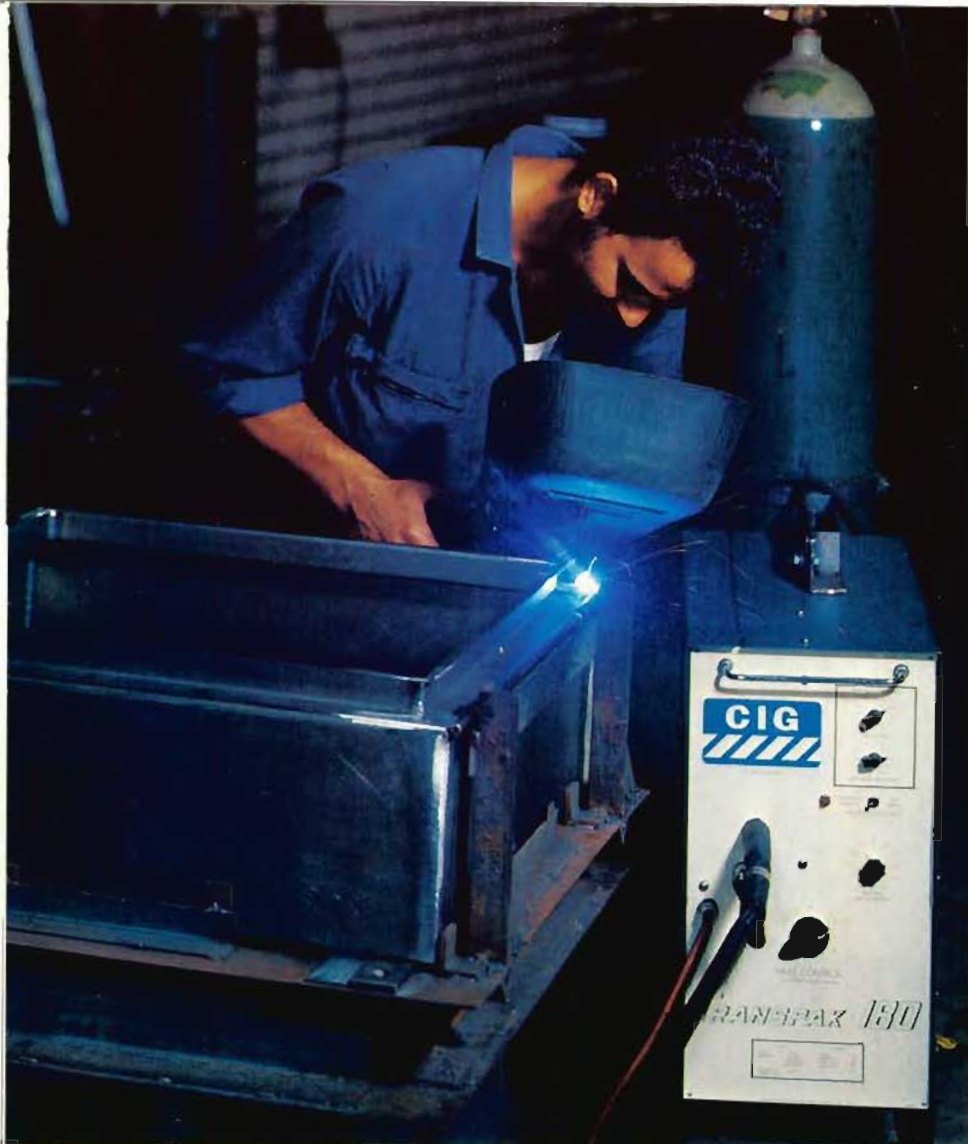
Transpak 180, latest machine developed by CIG for M.I.G. welding, is an ideal unit for sheet metal workshops.
