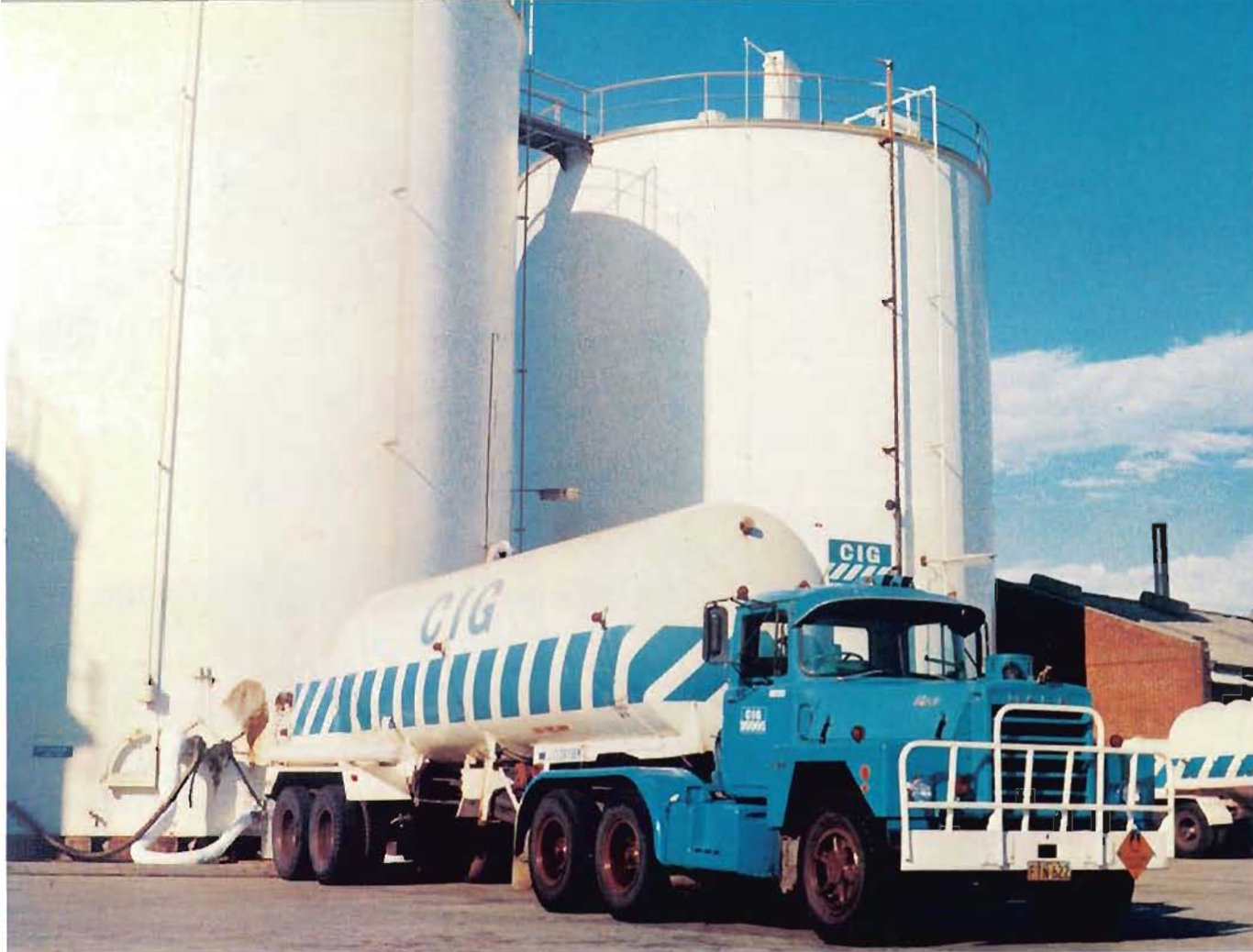
Liquid oxygen tanker being filled from storage tanks at C I G 's Sydney plant.
