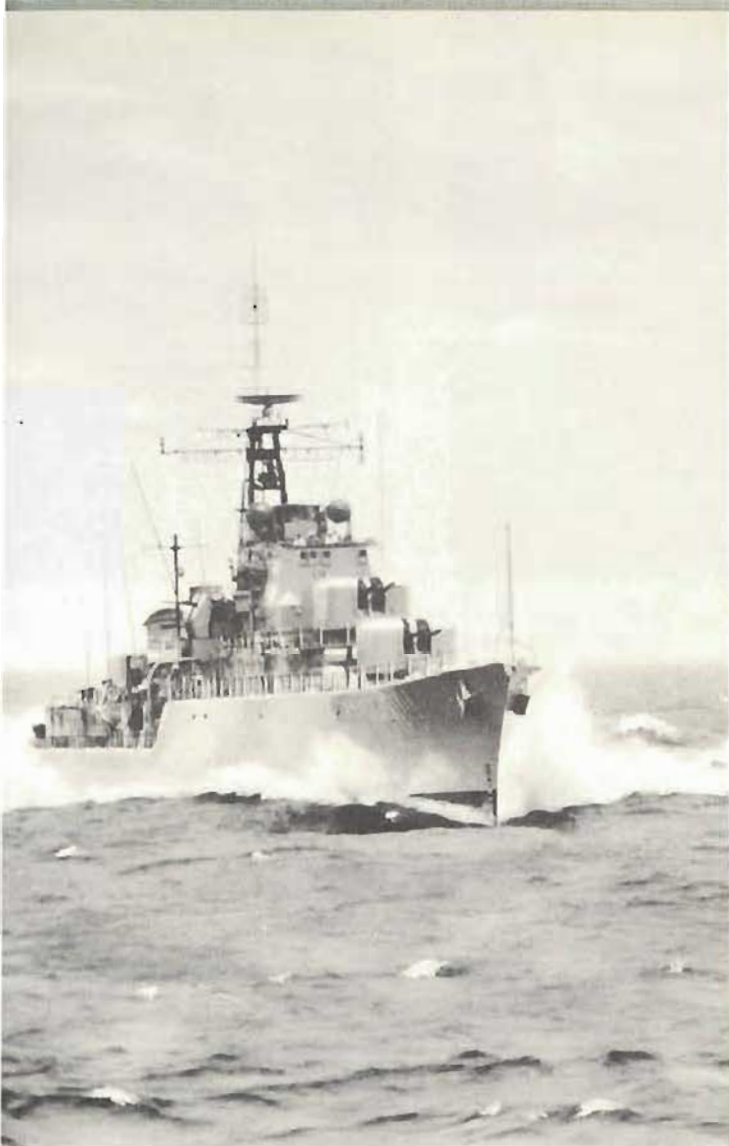
In 1957 H.M.A.S. Voyager became the first all-welded destroyer to be built in Australia. Aluminium was used extensively.
