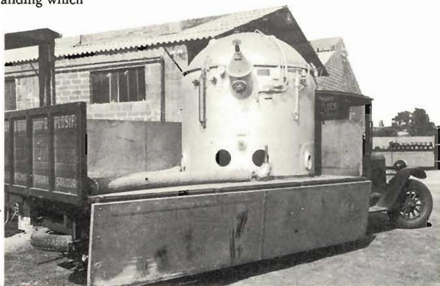
Early Heylandt tanker for the transport of liquid oxygen.
