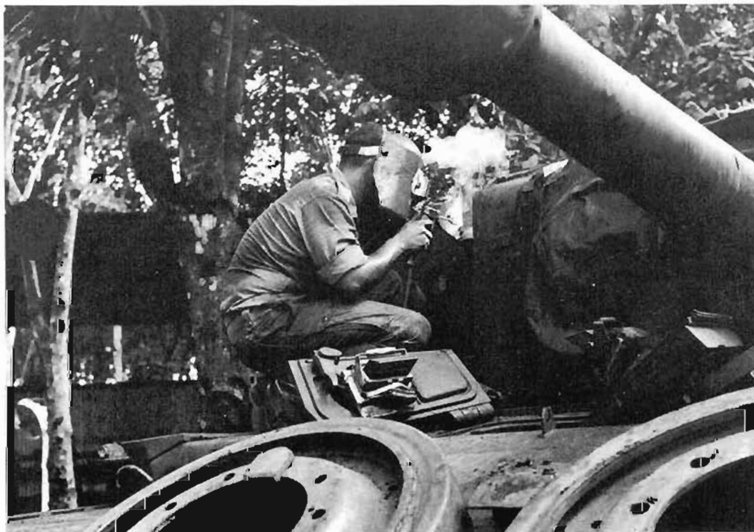
RAEME trooper repairing a Centurion tank with arc welder at Nui Dat, the Australian base in Vietnam.
