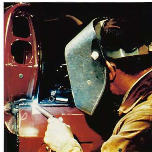
CIG's M.I.G. welding equipment being used in a car body repair shop.
