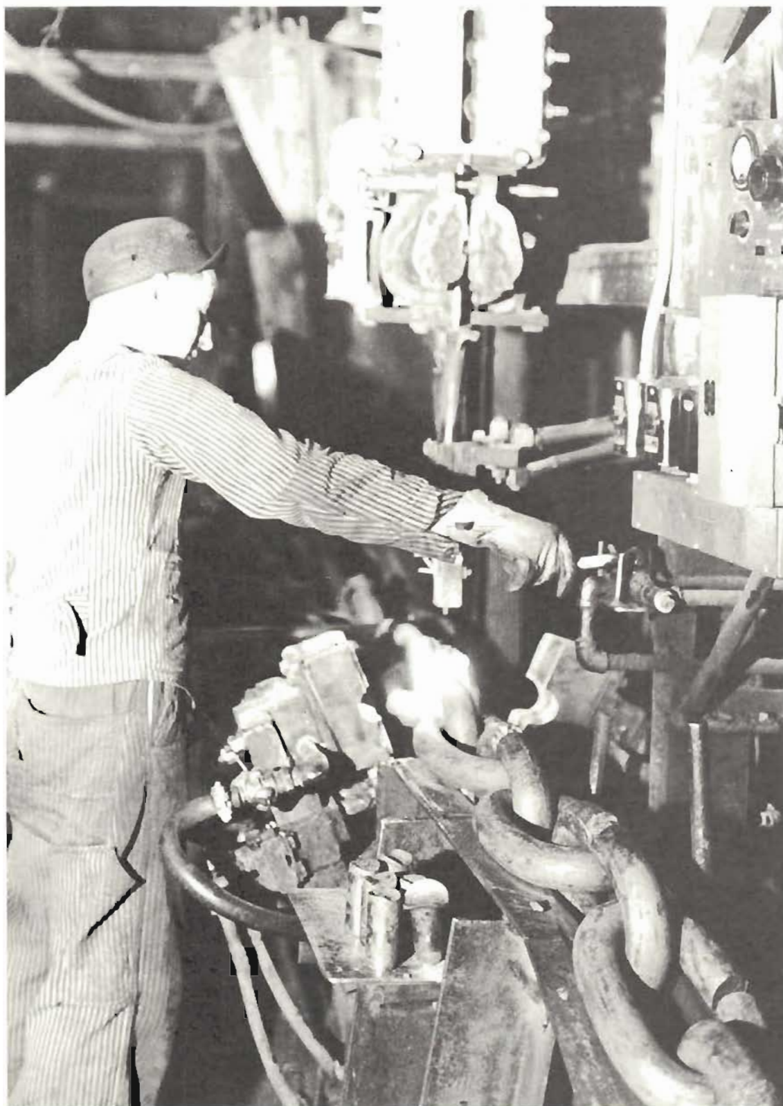
Technique for flash-welding anchor chain was evolved to assist N.S.W. Government Railways to meet R.A.N. order.
