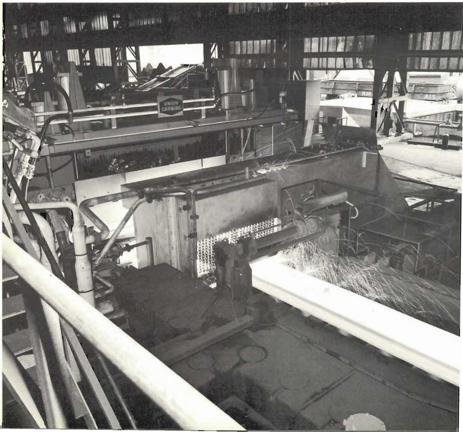
Automatic scarfing machine installed by C I G at Port Kembla steelworks.
