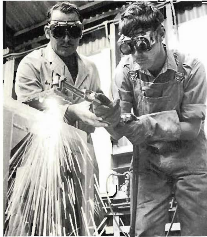
Army instructor guiding an apprentice in the use of oxy-acetylene cutter, an important military tool.
