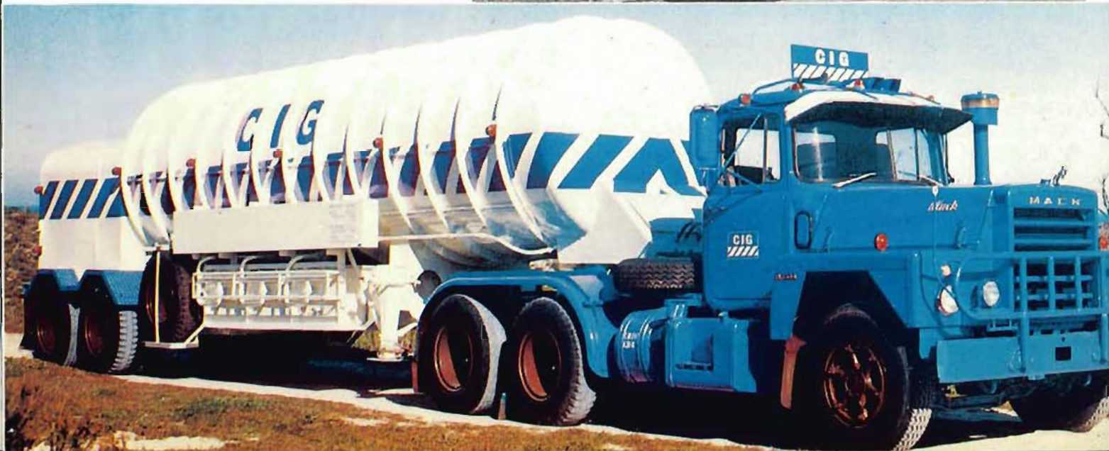
CIG tanker for long distance haulage of liquid oxygen. These vehicles supply Mount Isa, Darwin and Port Hedland.
