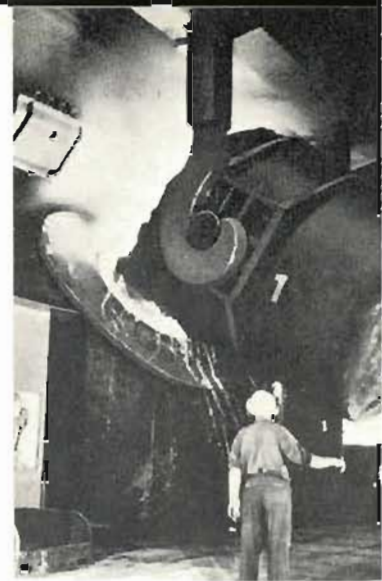
BOS furnace is tilted and charged with scrap. Transfer ladle is then emptied into it.
