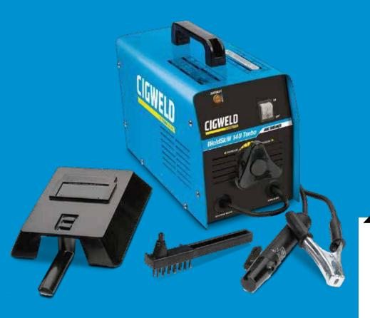
The CIGWELD Weldskill 140 Turbo is a fan cooled home arc welder that has a welding current range from 40 to 140 amps and is designed to operate from a 240V, 15 Amp power point. It will run standard general purpose 2.0mm electrodes for light gauge steel, generally less than 3.0mm thick, and up to 3.2mm electrodes for heavier sections.
